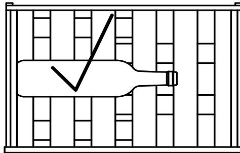
Note: When take the bottle out at the bottom of liner, move the bottle left or right. avoid display box removed. if forced to pull out, could result in damage to the bottom of the electrical box!
