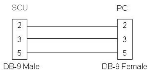
Figure 20. SCU RS-232 Pin Definition
