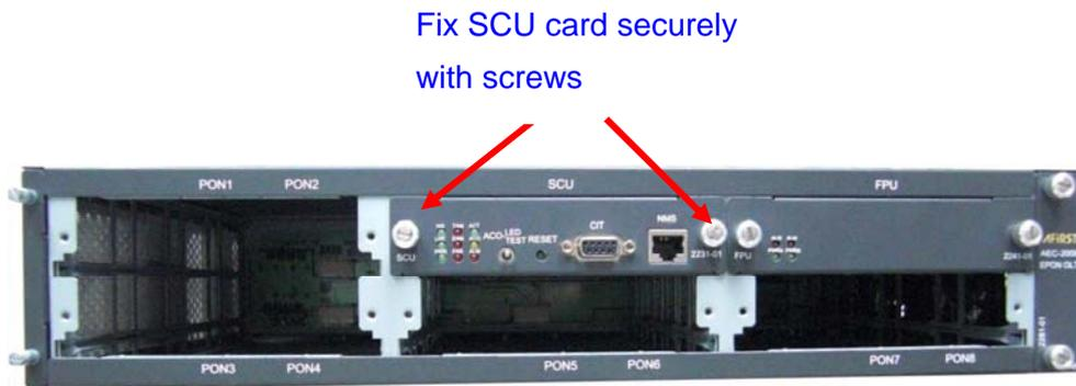
Figure 11. Installing SCU Card
