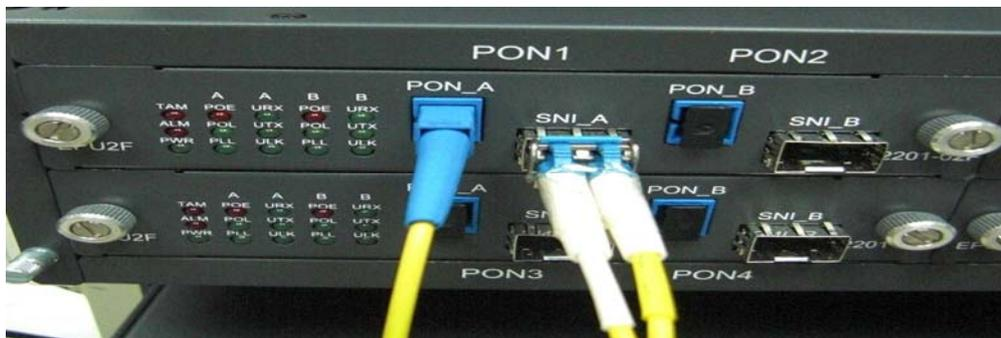
Figure 19. SNI Port Cable Connection
