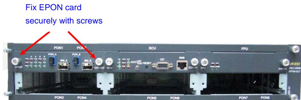
Figure 12. Installing Line Cards
