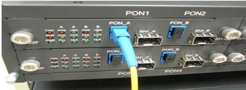
Figure 18. PON Port Cable Connection
