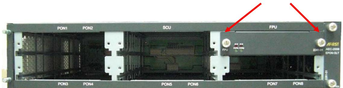
Figure 16. Installing FPU Card
