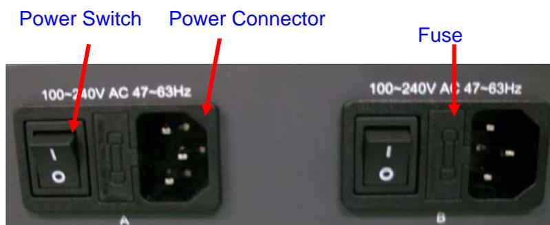
Figure 14. OLT Shelf AC Power Installation
