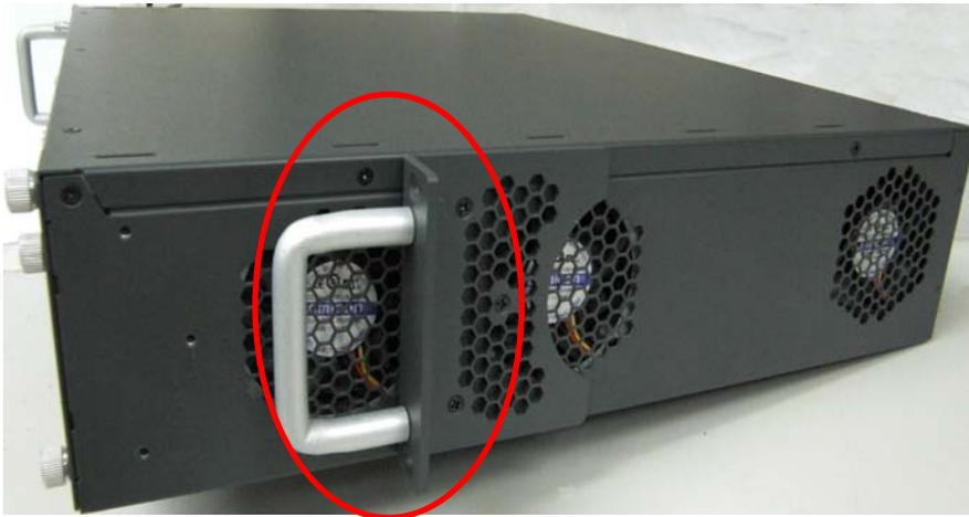
Step 2: Mount OLT-200 and fix with screws in the Rack
