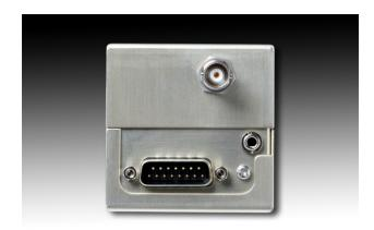
The XCOM VHF Transceiver has a 2.25" (57mm) face for fitting in a normal aircraft small instrument hole. The case is 5.1" (129mm) long, 2.4" (61mm) wide and 2.4" (61mm) high. The unit is secured to the aircraft dashboard by 4 screws and is self supporting, requiring no additional supports, trays or brackets.
