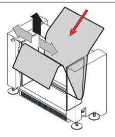
Align paper web to the left on the fixed stop page (max. 2mm/0.08" clearance).
