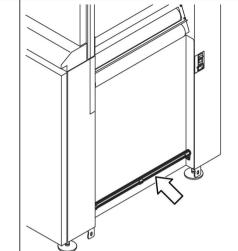
Use a vacuum cleaner to remove paper dust from the antistatic strip.
