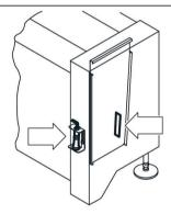
Use a soft cloth to clean the photo cell and reflector in the vacuum unit.
