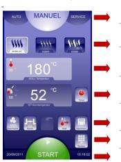
Select operating module: Manual = set cooking parameters manually: operating mode, temperature and time.
