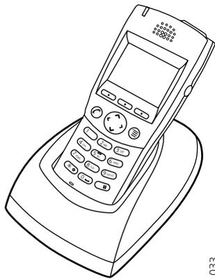
The Desktop Charger is used for charging your handset, for example at your desk. The tilted design facilitates the use of handsfree operation, e.g. in loudspeaking mode. The charger is delivered with a plug-in power supply and is connected into a wall socket.
