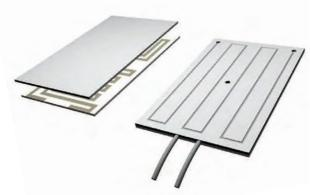
The AIN matrix is constructed of two parts. The heating element is printed on one of the AIN parts. Then, the parts are sintered together, making them one homogeneous assembly.
