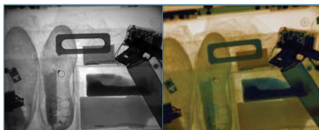
B/w image and image in dual energy mode of the same bag
