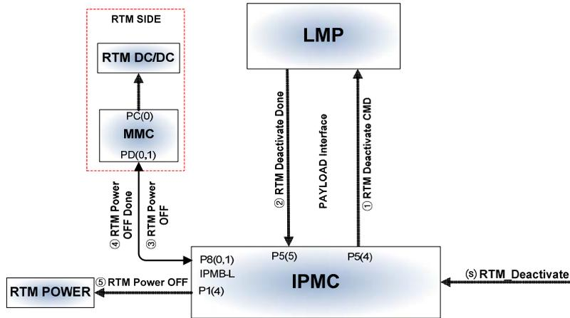
Figure 7-5 RTM Deactivate Procedure
