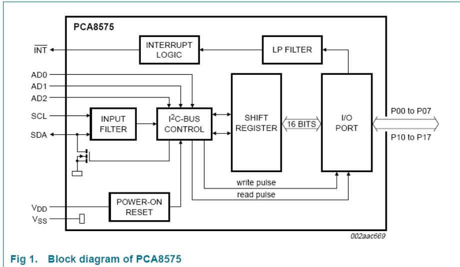
Fig 1. Block diagram of PCA8575
