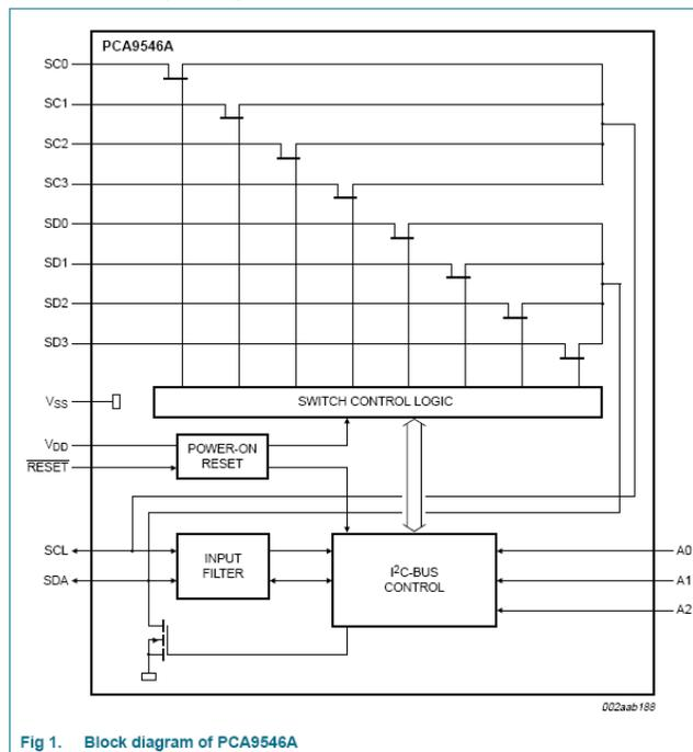
Fig 1. Block diagram of PCA9546A
