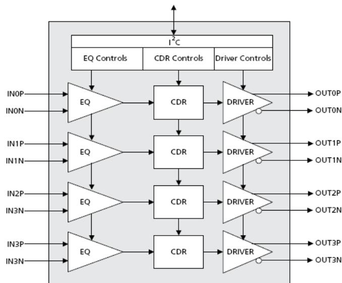
Figure 6-2 GN2405 Block diagram
