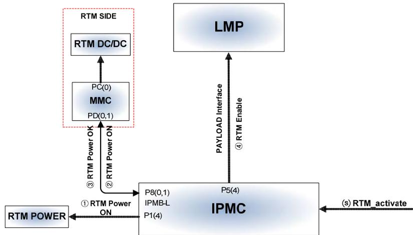
Figure 7-6 RTM Activate Procedure
