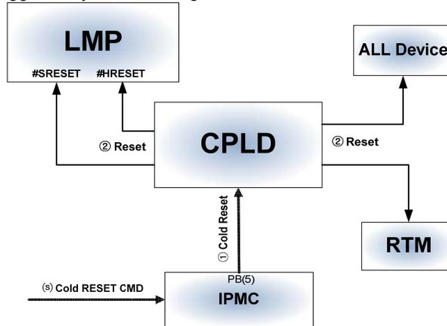
Figure 7-2 Cold Reset Procedure
