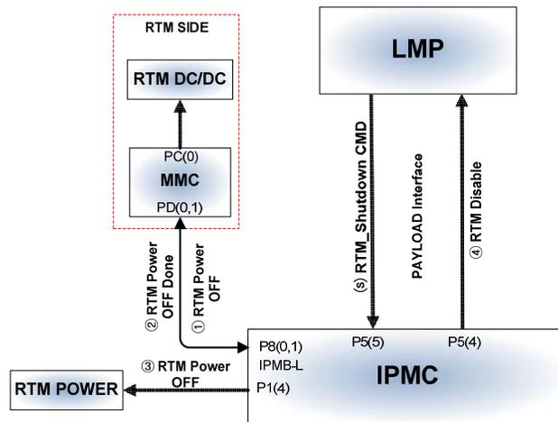
Figure 7-8 RTM Shutdown Procedure
