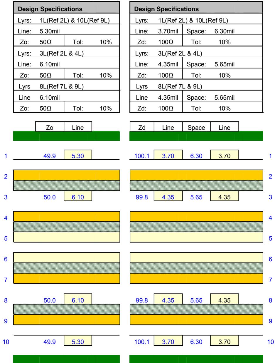
Figure 11-2 PCB Layer Stack-up
