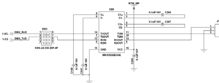
Figure 4-1 Header J1 and Switch SW1
