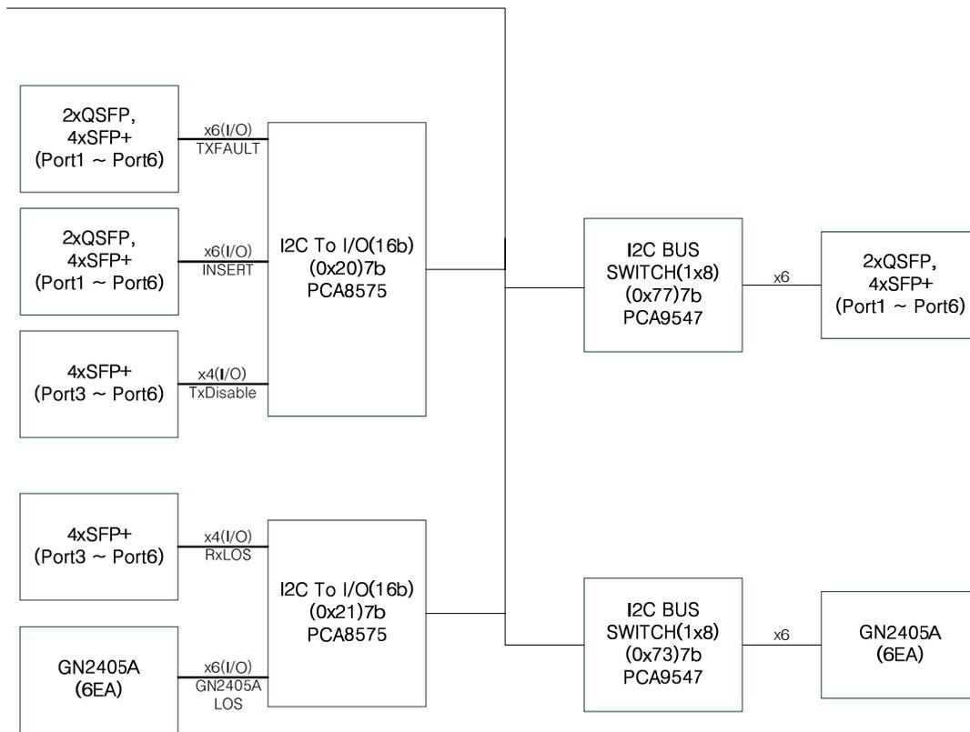
Figure 4-5 Devices on I2C Bus
