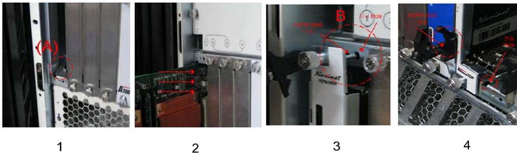
Figure 4-4 Plugging the Board
