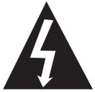
**THIS SYMBOL INDICATES THAT HIGH VOLTAGE IS PRESENT INSIDE. IT IS DANGEROUS TO MAKE ANY KIND OF CONTACT WITH ANY INSIDE PART OF THIS PRODUCT.**
