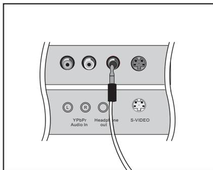
Plug a set of headphones into the 3.5mm mini-jack socket on the rear panel of the set.
