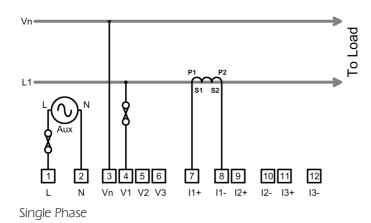
Where applicable V1(4), V2 (5), V3 (6) can be linked to L(1). A fuse must be used (see note above) from L supply to L(1)
