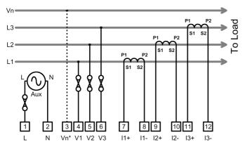
Ensure fuses are wired in as shown! A suitable Din rail mounting fuse holder is type CSFL4U (for fuse 1A 5 x 20mm fuse, not included) and end plate type CSFLEPU. Refer to Eltek.
