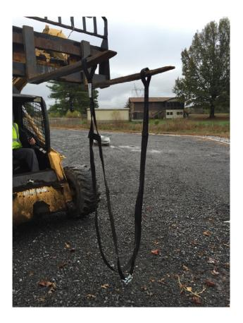
NOTE—The shackle is intended to go around the root ball on the side away from the machine so that you can disengage the B&B Tree Buddy without removing it from the forks after the tree is planted.
