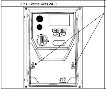
Using a suitable flat blade screwdriver, rotate the two retaining screws indicated until the screw slot is vertical.
