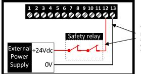
Wires should be protected against short circuits as shown above
