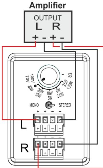
Figure 2: Yarden 6-OD Stereo Setup
