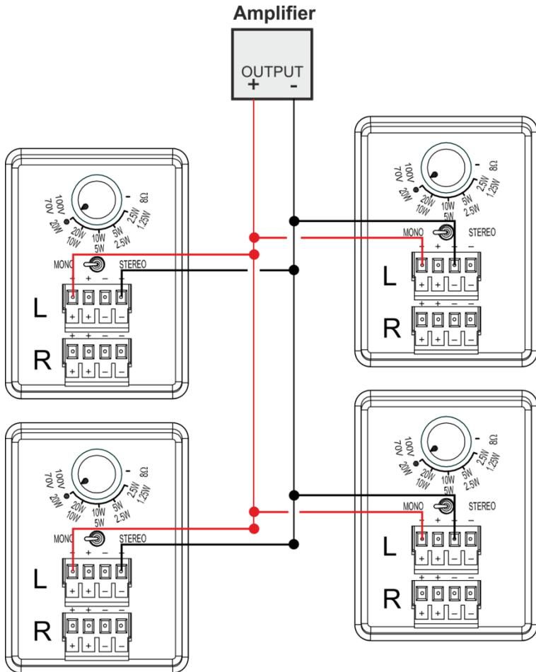
Figure 7: Square Layout Parallel Wiring
