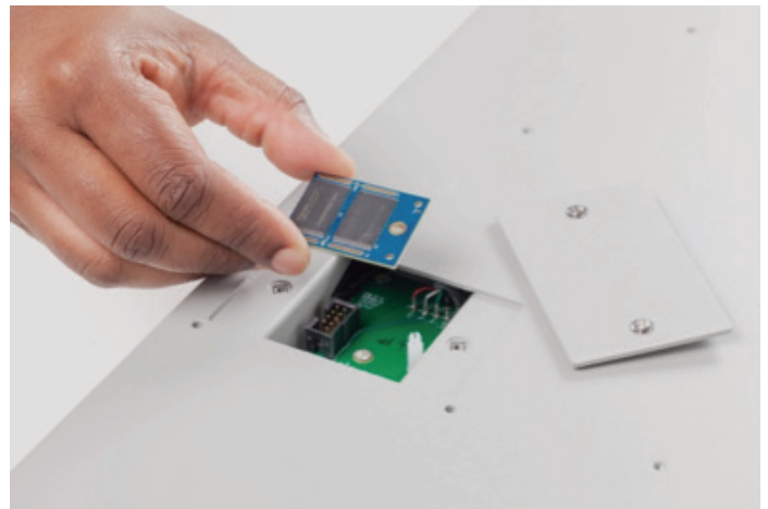
Figure 3. Installing the N7908A BBR hardware option on an APS power supply
