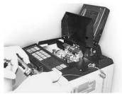
9. Optical Fiber Splicing Check the color of fibers and remove coatings. Cut the fiber using an approved fiber cutting method. Splice fibers using an approved fiber splicing method.
