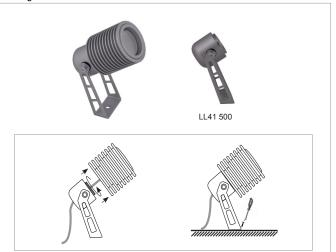
1.4.1 The power cable string on bracket. The bracket screw on the basic unit. Connect the fixture to AC power supply and fix the bracket with screws to the surface.
