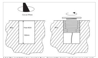
1.3.1 The installation box insert in floor. Connect the basic unit to power supply and put the fixture in the box. Screw the front cover.
