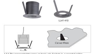
1.2.1 The recessed holder screw on basic unit. Cut hole in suspended ceiling. The aloved thickness of ceiling material is max. 12mm.
