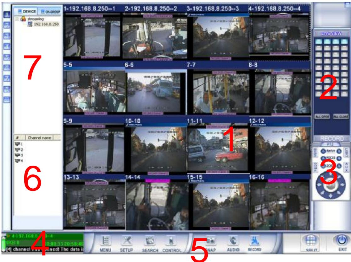
1. **Image Display Windows:** Display maximum 16 channels. The displayed channel quantity can be changed by click split icon in the corner of the main interface.
