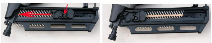
Unload the nail strip by press the nail stopper and slide out the nail strip.
