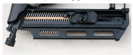
• To unload the fastener from the magazine, press the release lever on the pusher and tilt the tool to slide the nail strip to the rear of the magazine.
