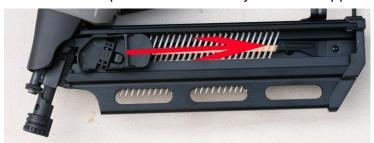
• Release the pusher to engage the nail strip and feed it into the nozzle.
