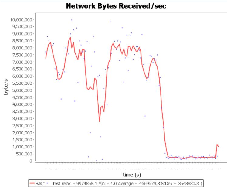
**Network Bytes Received/sec:** this diagram shows the speed of server received data from the network during the measurement interval. The units of the speed are bytes per second.
