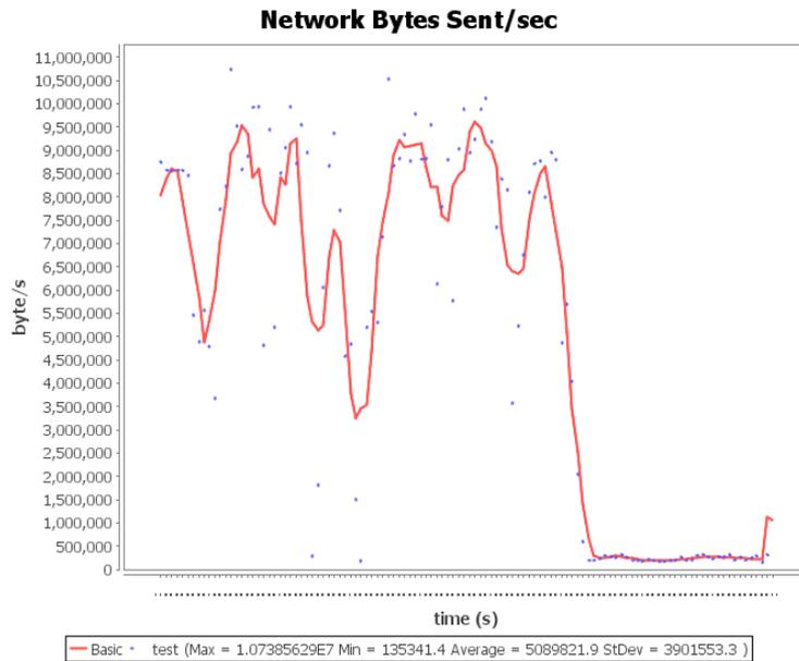
**Network Bytes Sent/sec:** this diagram show the speed of server sent data to the network during the measurement interval. The units of speed are bytes per second.
