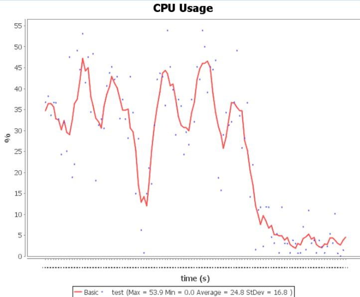
**CPU Usage:** this diagram shows the CPU Usage of the server during the measurement interval.
