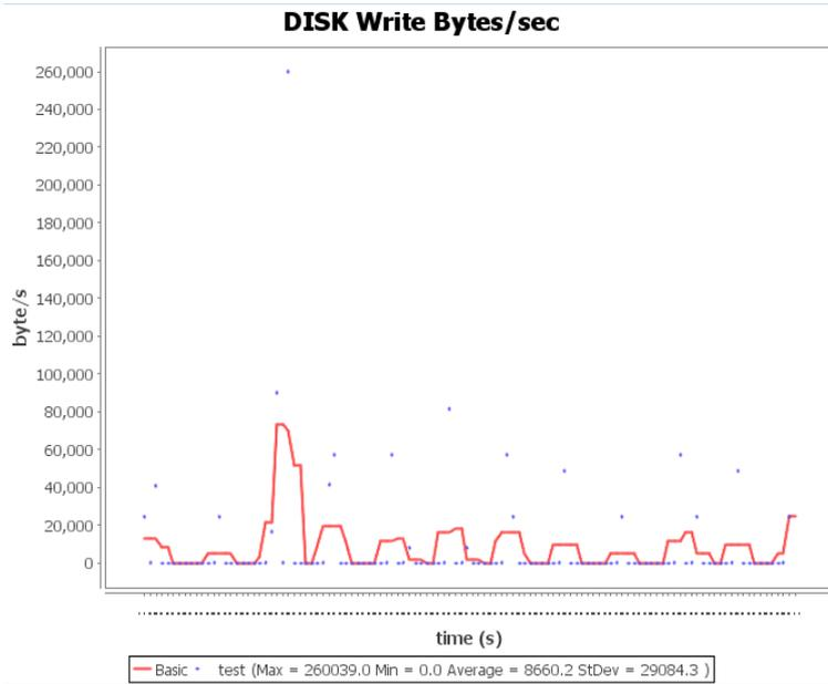
**DISK Write Bytes/sec:** this diagram shows the speed of disk write during the measurement interval. The units of the speed are bytes per second.
