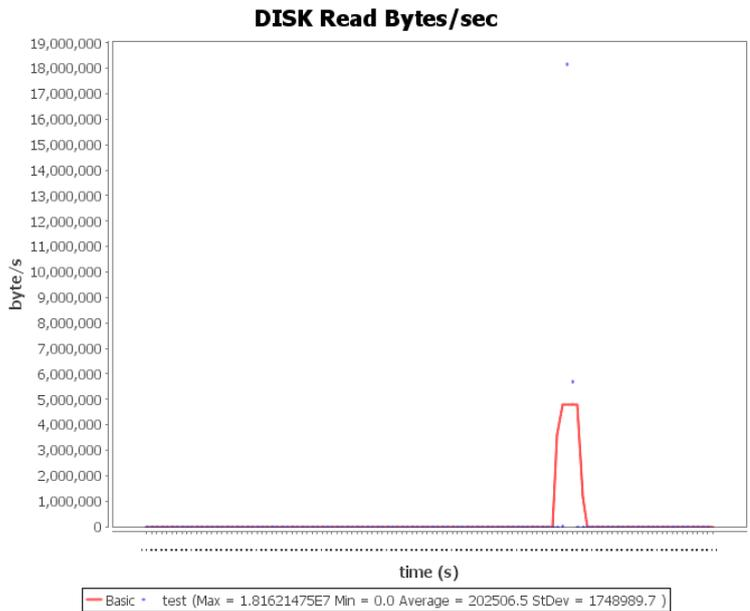
**DISK Read Bytes/sec:** this diagram shows the speed of disk read during the measurement interval. The units of the speed are bytes per second.
