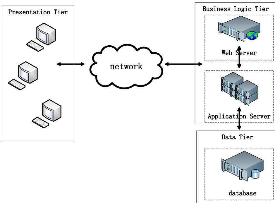
SUT (System Under Test) contains the business logic to simulate the tested scenario. The SUT comprises all components which are part of the “application” being simulated. This includes network connections, Web Servers, application servers, database servers, etc. The SUT of Bench4Q is based on a distribution of the TPC-W Benchmark Java Implementation originated of PHARM at the University of Wisconsin - Madison.
