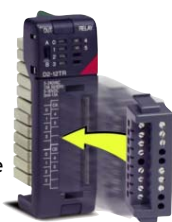
16-point module with removable terminal block
