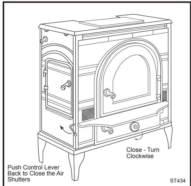
Fig. 22 Closing the primary and underfire air supply.
