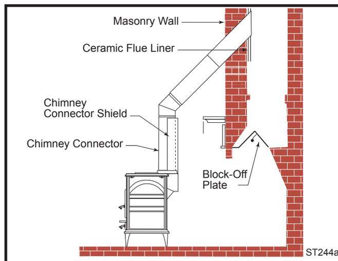
**Fig. 8** The connector enters flue above the fireplace. If the clearance between the chimney connector and either the mantel and/or the ceiling is inadequate, special protective shields will be required.
