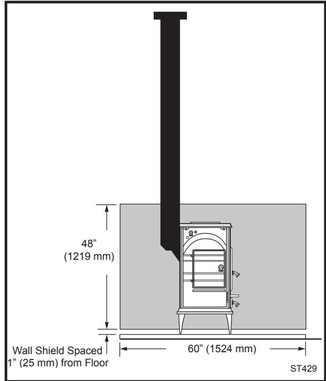
Fig. 17 Sidewall protection.
