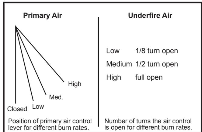
Fig. 24 Primary and Underfire air settings.
