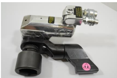
Torque with reaction arm
