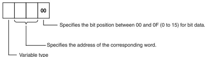
Word addresses for specific memory area words can be calculated by converting the normal decimal word address to hexadecimal and adding it to the first word in the *Addresses for communications* column in the above table. For example, the address for communications for D00200 would be 0000 (from above table) plus C8 (decimal 200 converted to hexadecimal), or 00C8.
