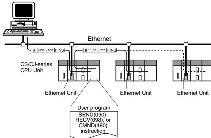
Executing, from the host computer, FINS commands with UDP/IP or TCP/IP headers enables various control operations, such as the reading and writing of I/O memory between PLCs, mode changes, and file memory operations.
