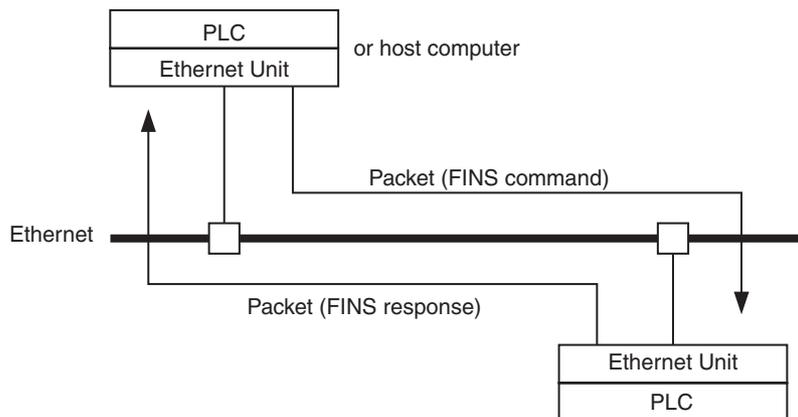
In the FINS communications service, both an IP address for IP (the Internet layer) and a FINS node address for FINS (the application layer) are used for the remote device. Also, 9600 is used as the default setting for the local UDP or TCP port number (i.e., the transport layer) for identifying the application layer, i.e., the FINS communications service. (Another number can be set for the FINS/UDP port from the Setup Tab in the Unit Setup.)
