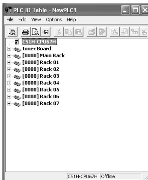
3. Read the I/O tables from the PLC and select the Rack to which the Ethernet Unit is mounted.
