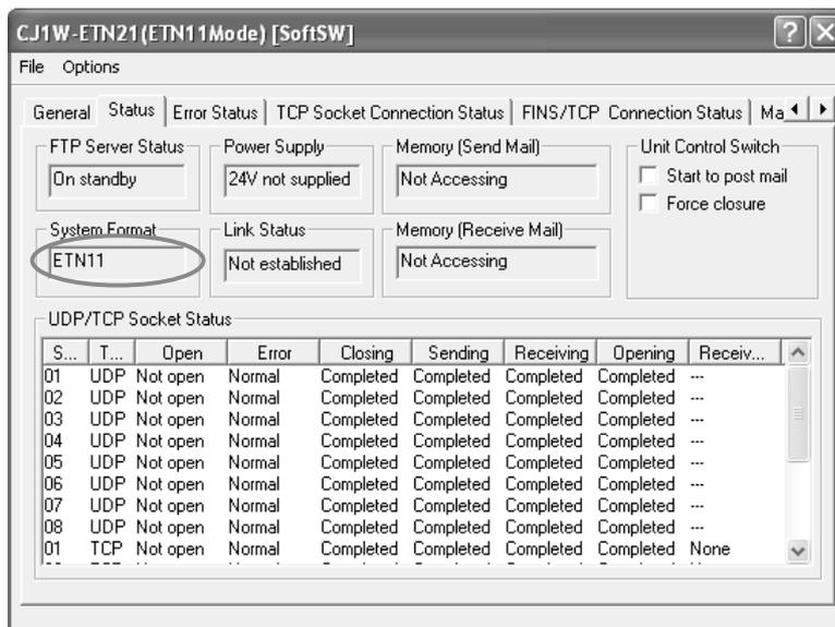
Checking with the CX-Programmer's Unit Setup Window
