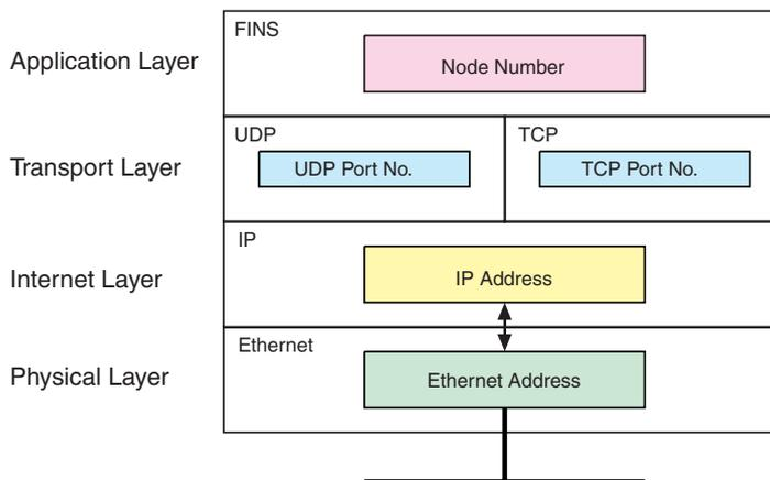
The FINS communications service is a communications method based on UDP/IP, and it is supported by most OMRON Ethernet-related products. (In this manual it is called the FINS/UDP method.) In addition to supporting the FINS/UDP method, the CS1W-ETN21 and CJ1W-ETN21 support FINS communications using TCP/IP. (In this manual, this is called the FINS/TCP method.)
