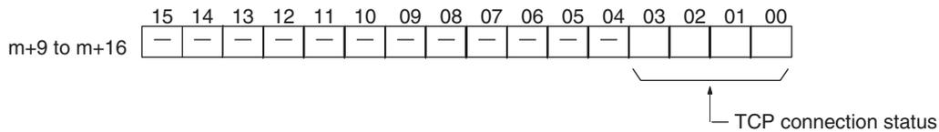
The connection status for each TCP socket is stored by code in this word. For details, refer to *Appendix C TCP Status Transitions*.
