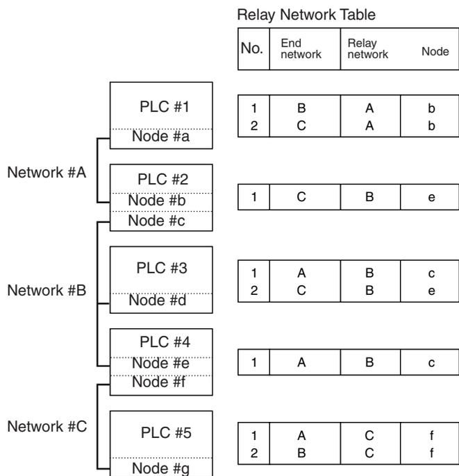
In the table for PLC #3, for example, if network #A is taken as the end network, then network #B becomes the relay network and node #c becomes the relay node. If network #C is taken as the end network, then network #B still becomes the relay network and node #e becomes the relay node.
