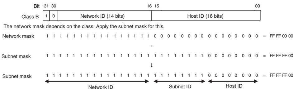
Set the same subnet mask value for all of the nodes on that subnetwork. If a subnet mask is not set (default setting of 0.0.0.0) or if an illegal value is set, the following subnet mask values will be used depending on the class of the local IP address.
