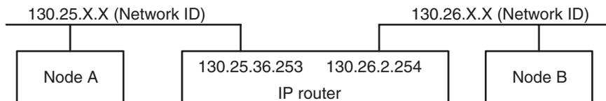
For the IP network address, set the network number (i.e., the net ID) of the other IP network segment with which communications are to be executed. The length of the network number (i.e., the number of bytes) will vary depending on the IP address class. Four bytes are reserved for setting the IP network address, so set the network number from the beginning and then set 00 in the remaining space.
