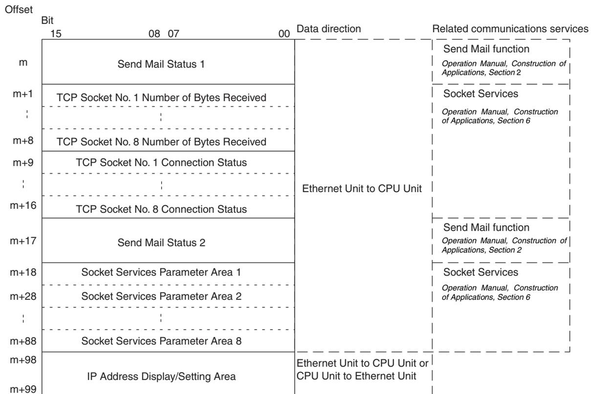
The meanings of the items shown in the above diagram are explained on the following pages. For details regarding the related communications services shown in the diagram, refer to the indicated sections.
