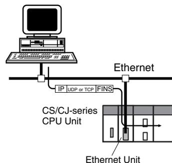
The FINS gateway function enables access to PLCs on not only the same Ethernet network but on various other networks, including SYSMAC LINK and Controller Link.
