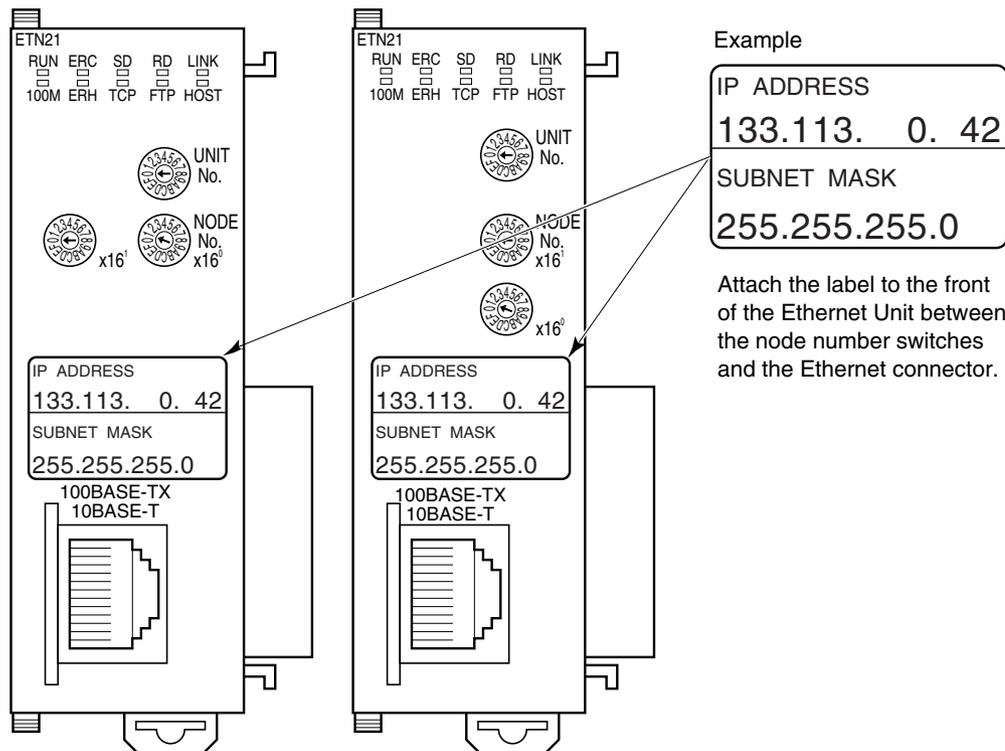
Each communications device connected to the Ethernet network is allocated a unique Ethernet address. For the Ethernet Unit, this Ethernet address is shown on the right side of the Unit as a 12-digit hexadecimal number.
