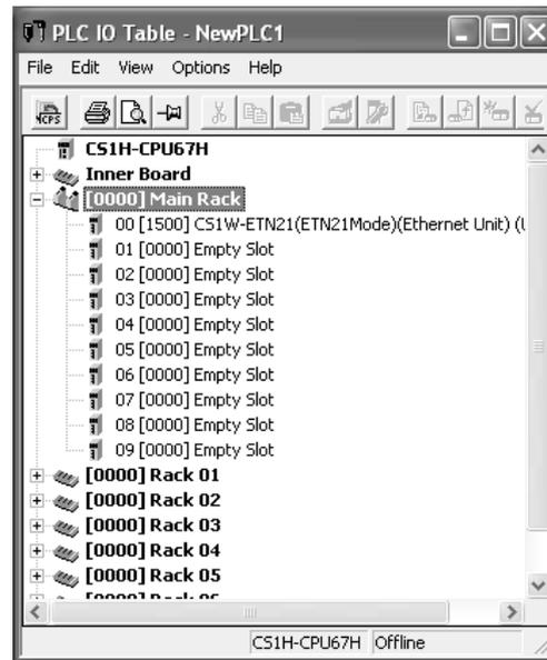
4. Move the cursor to the Ethernet Unit and right-click. Select *Unit Setup* from the popup menu to display the window for making the Ethernet Unit Setup. The default settings are shown below.
