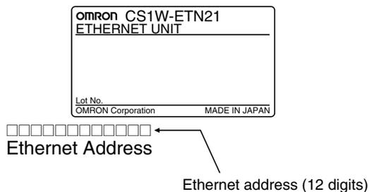
**Note** The Ethernet address can also be checked using the FINS command, CONTROLLER DATA READ. For details, refer to 7-3-2 CONTROLLER DATA READ on page 162.
