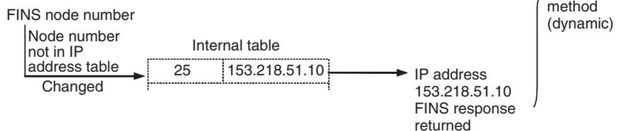
**Note** When an internal table IP address has been changed with the reception of a FINS command, this is sent to the IP address in the internal table.
