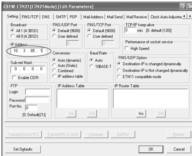
When an IP address is set in the Unit Setup, that value is displayed in the IP Address Display/Setting Area in the DM Area words allocated for CPU Bus Units.
