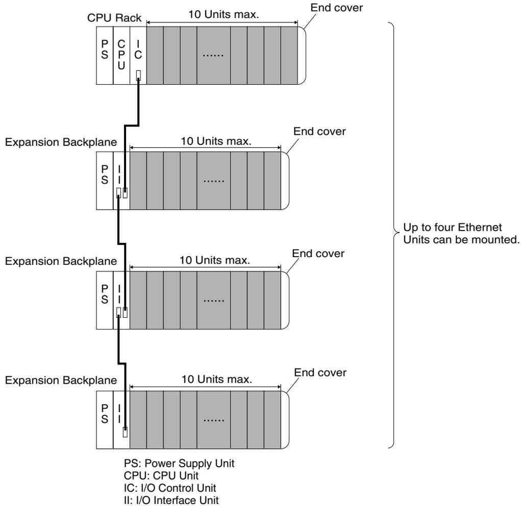
The CJ1W-ETN21 Ethernet Unit's maximum current consumption is 370 mA. Make sure that the total current consumption of all the Units connected to the same CPU Backplane or Expansion Backplane does not exceed the output capacity of the Power Supply Unit.
