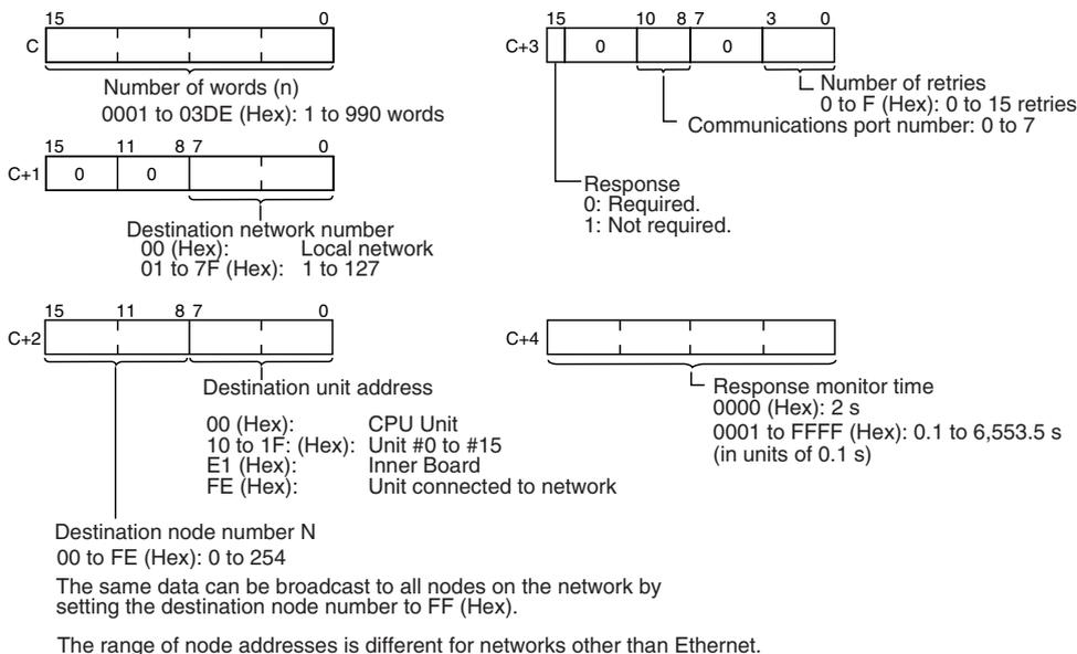
**Note** The message service does not guarantee that a message will reach the destination node. A message may be lost during transmission due to factors such as noise. To prevent this from occurring when using message services, it is common to set up retry processing at the node from which instructions are issued. With the SEND(090), RECV(098), and CMND(490) instructions, retry processing is executed automatically by specifying the number of retries, so specify a number other than 0.
