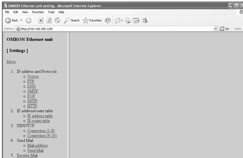
3. Select **1. IP address and Protocols - System** to display the *Login Password* field on the right of the window.
