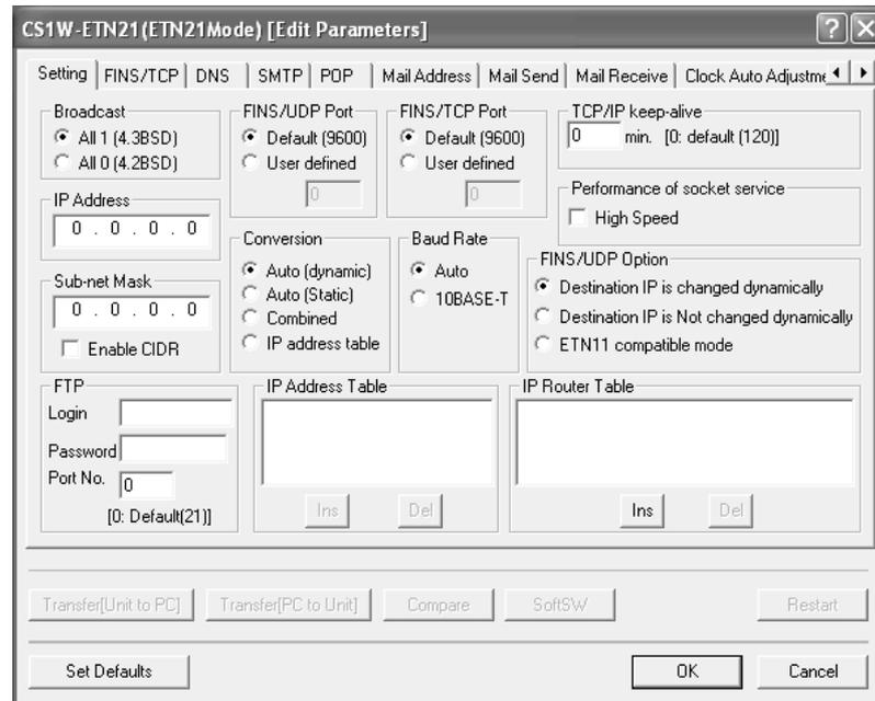
At the point where the Ethernet Unit is mounted and the I/O tables has just been created, the default values are in effect for all of the settings.
