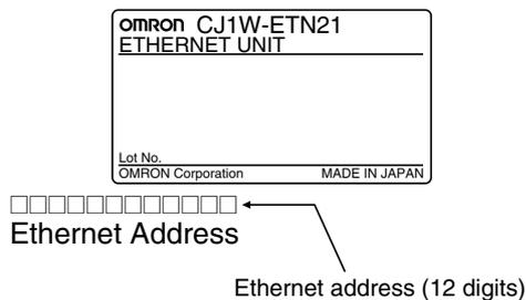
**Note** The Ethernet address can also be checked using the FINS command, CONTROLLER DATA READ. For details, refer to 7-3-2 CONTROLLER DATA READ on page 162.
