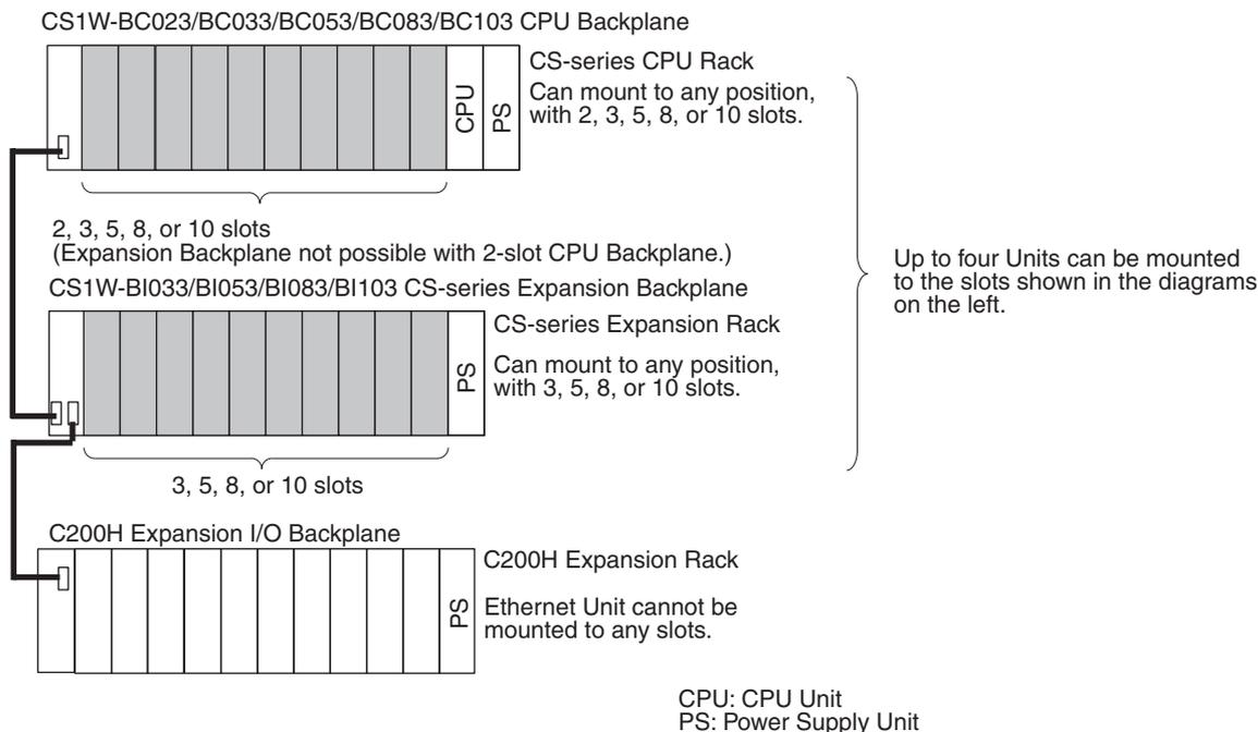
**Note** The CS1W-ETN21 Ethernet Unit's maximum current consumption is 380 mA. Make sure that the total current consumption of all the Units connected to the same CPU Backplane or Expansion Backplane does not exceed the output capacity of the Power Supply Unit.
