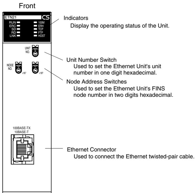
Each communications device connected to the Ethernet network is allocated a unique Ethernet address. For the Ethernet Unit, this Ethernet address is shown on the right side of the Unit as a 12-digit hexadecimal number.
