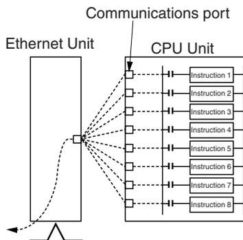
There are eight communications ports, so up to eight communications instructions can be executed at a time. The number of messages that can be sent or received with a single CPU Bus Unit service, though, is not more than two each for the CPU Unit to the Ethernet Unit and for the Ethernet Unit to the CPU Unit.
