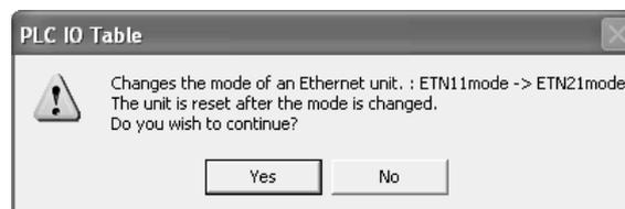
3. After the mode has been changed, the following confirmation message will be displayed. Click **OK** to restart the Ethernet Unit. After the Unit has been restarted, it will begin to operate in ETN21 mode.
