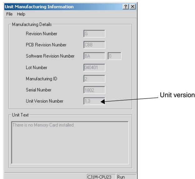
Use the above display to confirm the unit version of the Unit connected online.
