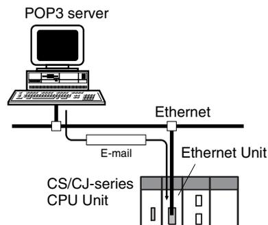
The following types of commands can be sent to the PLC: I/O memory read and write, backup, operating mode changes, and file transfers (of 1 Mbyte or less).
