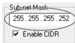
If CIDR is not enabled and a subnet mask is not set (i.e., the default of 0.0.0.0 is set) or an illegal value is set, one of the following values will be set as the network mask according to the class of the local IP address.
