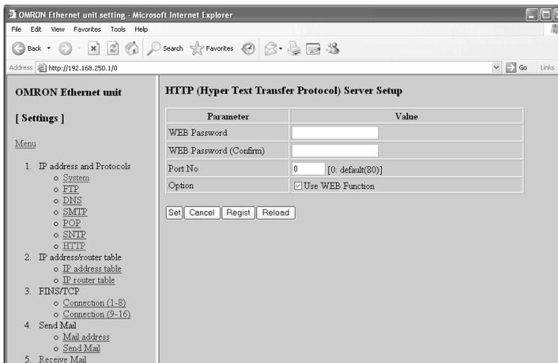
6. Make the required settings (i.e., the password in this example). To prevent incorrect password entry, set the same password in the *WEB Password* field and *WEB Password (Confirm)* field.
