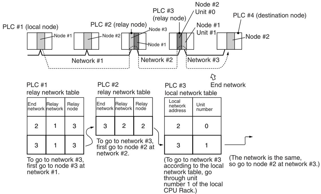
**Note** In the above example, the routing tables required for a message to reach PLC #4 from PLC #1 are shown. Additional settings would be required in the routing tables for a message to reach PLC #1 from PLC #4. Refer to 6-4-3 *Routing Table Setting Examples* for routing table setting examples.
