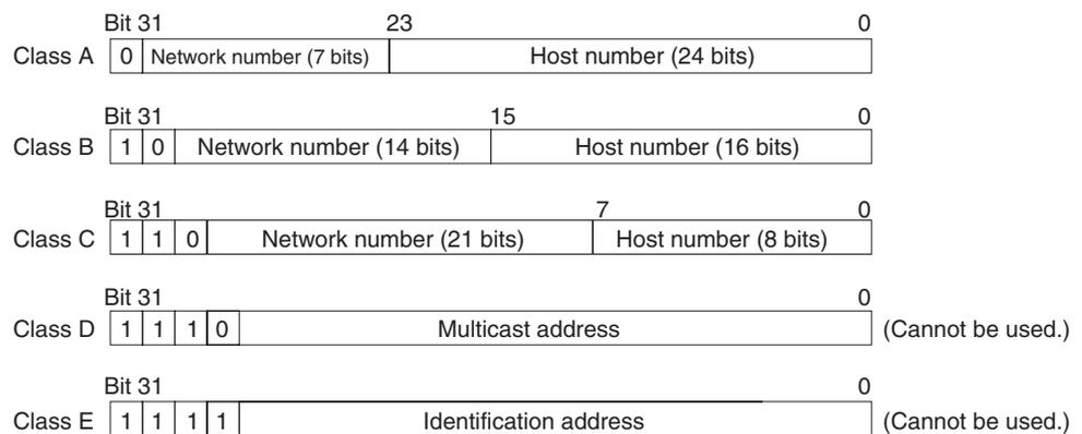
The number of networks in each class and the number of nodes possible on the network differ according to the class.
