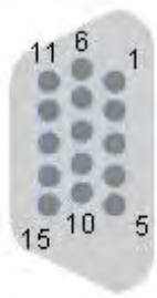
Figure 1.5 CN1 pin definition
