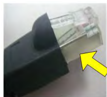
Figure 1.2 Connector with Metal Shielding
