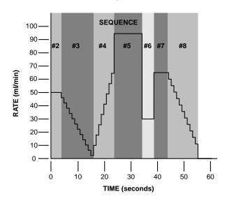
Here is an example of a more complex profile program. Each "run" of the infusion has been determined to pump 43.155 ml. The first sequence refills the syringe with the volume to be infused then the infusion profile is started, after which the syringe is refilled and the infusion is repeated until the pump is stopped.
