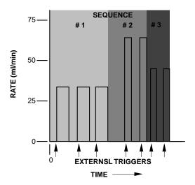
Here, a series of dispenses are programmed. Each dispense is started by a trigger, such as pressing the RUN/STOP key or pressing an attached foot switch. Seven dispenses are programmed: three of 15 ml at 35 ml/mn, two of 25 ml at 65 ml/mn, and two of 17 ml at 45 ml/mn. The pump's display will show "TRIGGER" when it is waiting for a run trigger and the Run LED will be off.
