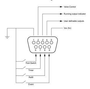
TTL Connections are via a 9 pin D-sub type connector. All inputs are internally pulled up to a logic high.
