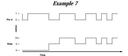
Before the pumping flow begins, the pump sends a TTL signal to another piece of equipment for 5 seconds, but first verifies that the TTL line is low by turning it off for 1 second, then turns it on.
