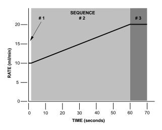
In this example, the pump will ramp up from 10 ml/mm to 20 ml/mn over 60 seconds, then continue to run at 20 ml/min for another 10 seconds. This is a Strategy 2 Program requiring four sequences:
