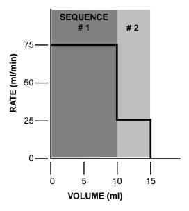
The following program will instruct the pump to infuse according to the above graph. The program instructs the pump to infuse 10 ml at 75.000 ml/mn then infuse another 5 ml at 25 ml/mn then stop, for a total of three sequences. Since this graph is Rate vs. Volume, Strategy 1 will be used when entering the program.
