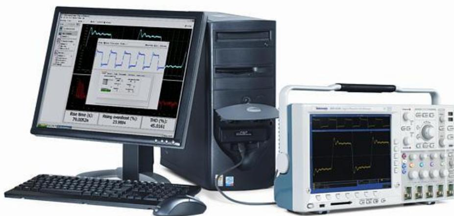
*Figure 4.1: Example showing a LabVIEW program controlling and displaying the oscilloscope's functions on a PC [NI].*
