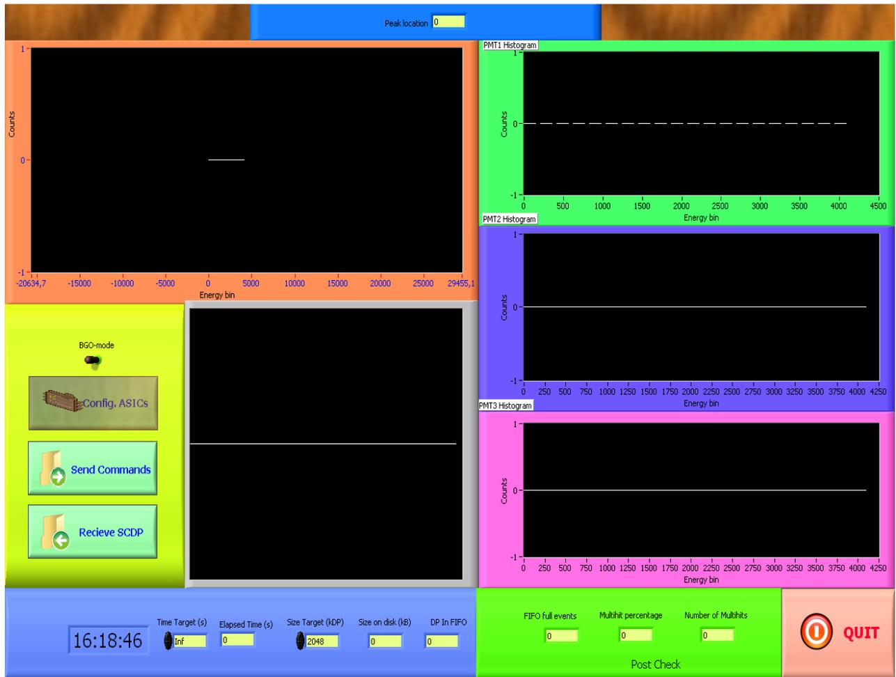
Figure 6.3: The Front Panel view of the main program in case of the BGO detector mode.
