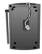
Connect the telephone line cord to the base (Step 3)
