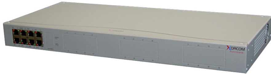
Figure 7: Atribank with 8 FXO Ports
