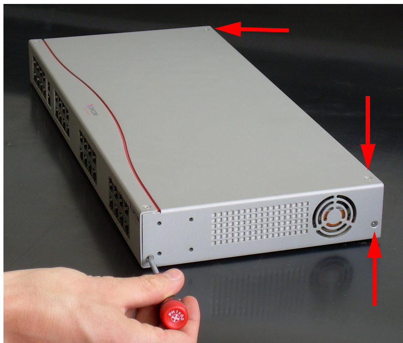
Figure 14: Removing the Six Screws (two on the far side are not pictured)
