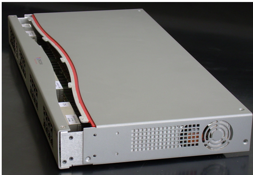
Figure 15: Removing the Cover
