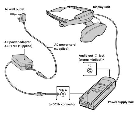
\* You can connect an optional headphone set. When using an optional headphone set, the sound from the Glasstron earphones is muted.
