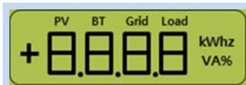
Here we can check the voltage, power, SOC or the current from the PV, Battery, Grid or the house consumption.
