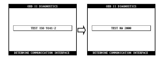
When succeeded in communicating with the control module with any of these 4 standard protocols, ULTRASCAN P1 reports the successful establishment of communication and waits for your command to commence generic OBD2 diagnosis as below:
