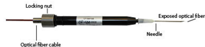
Adjustment of the fiber position.
