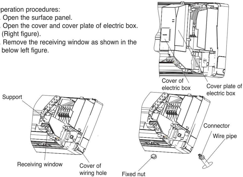
4. Wire pipe should be tightened by the fixed nut and the electric box should be fixed as shown in the above right figure and the below figure.
