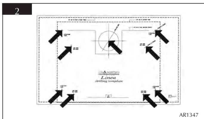
TAKE CARE WHEN MARKING OUT THE FLUE AS IT IS VERY DIFFICULT TO MOVE AFTER INSTALLATION.
