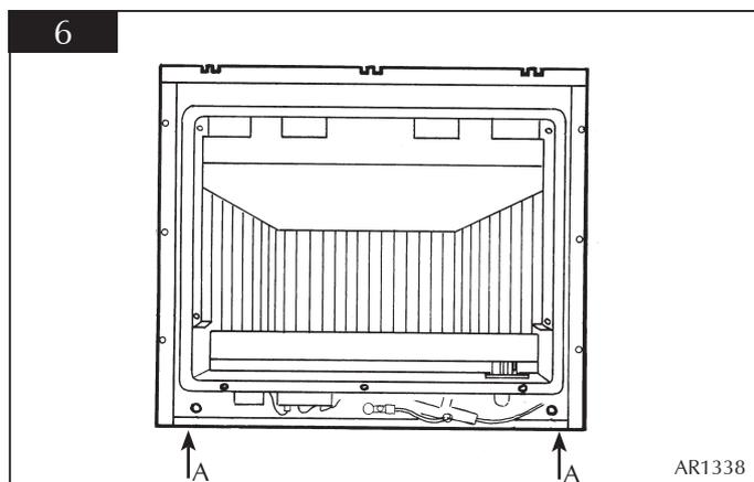
**DO NOT OVER TIGHTEN. DO NOT DEFORM THE REAR OF THE APPLIANCE.**
