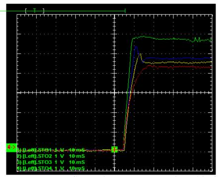
Startup transients. Center line is moment of Enable ON.
