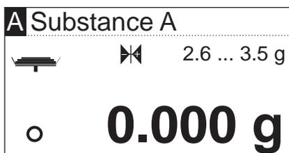
The display shows the target weight for the sample that has been specified for the corresponding method (in this example for "substance A"). Rather than having any effect on the measurement process, this target weight just serves as a weighing-in guide. To obtain the best possible reproducibility of results, the sample quantity weighed in should lie within the target weight tolerances.
