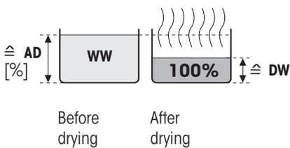
The wet weight of the sample is displayed (and printed out) as a percentage of the dry weight (= DW = final weight = 100%). When the results are printed out, the ATRO dry content is designated “%AD” (ATRO Dry Content) (e.g. 312.56 %AD). During the drying the current measured value is continuously displayed in percent.
