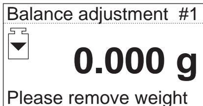
After a short time you will be asked to remove the adjustment weight. Remove the weight from the sample pan.
