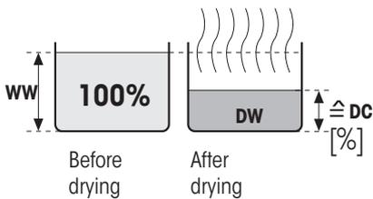
The dry content of the sample is displayed (and printed out) as a percentage of the wet weight (= ww = initial weight = 100%). When the results are printed out, the dry content is designated “%DC” (Dry Content) (e.g. 88.65 %DC). During the drying the current measured value is continuously displayed in percent.
