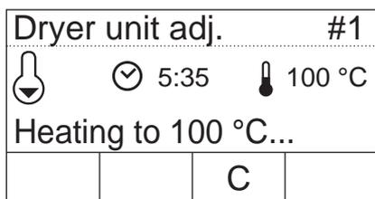
The heating module is heated to a temperature of 100 °C. You can follow this process on the temperature display. The instrument now waits 15 minutes until the temperature adjustment set shows the correct temperature, a beep is then given.
