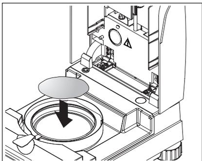
Place the provided specimen sample in the sample pan.
