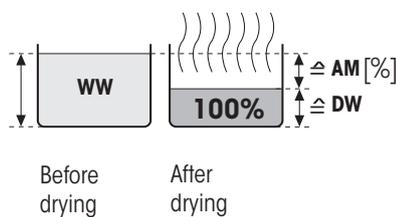
The moisture content of the sample is displayed (and printed out) as a percentage of the dry weight (= DW = final weight = 100%). When the results are printed out, the ATRO moisture content is designated “%AM” (ATRO Moisture Content) (e.g. -255.33 %AM) and shown as a negative value. During the drying the current measured value is continuously displayed in percent.
