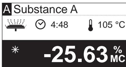
When drying is complete, an audio signal sounds and the bottom section of the display is shown in inverse (white font on dark background).
