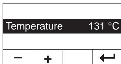
The current drying temperature flashes. You can use the «+» and «-» keys to change the temperature in the range from 50 to 200 °C in 1 °C increments. **Note:** If you choose a drying temperature of over 160 °C, for reasons of backward compatibility with methods already developed for the Moisture Analyzer HB43, you can choose timed temperature reduction.
