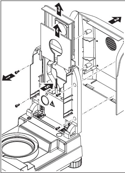
To dismantle the heating module the four screws (1) must be unscrewed. A screwdriver is needed for this purpose (Torx T-20).
