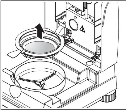
Carefully remove the sample pan handler from the sample chamber.
