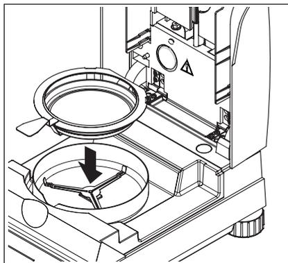
Position the empty sample pan in the sample pan handler. Place the sample pan handler in the draft shield. Ensure that the tongue of the sample pan handler lies exactly in the slot of the draft shield. The pan must lie flat in the pan holder.
