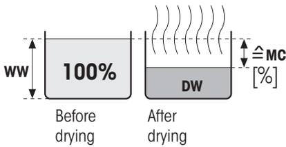
The moisture content of the sample is displayed (and printed out) as a percentage of the wet weight (= ww = initial weight = 100%). This is the factory setting. When the results are printed out, the moisture content is designated “%MC” (Moisture Content) (e.g. -11.35 %MC) and shown as a negative value. During the drying the current measured value is continuously displayed in percent.
