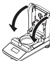
Close the heating module and the instrument then automatically begins the drying and measuring process.
