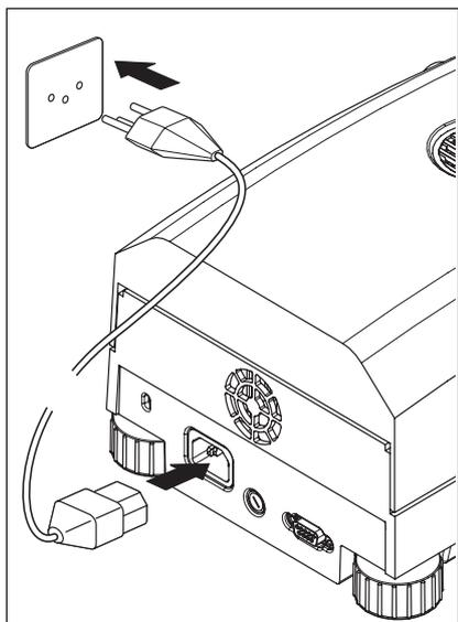
Connect the instrument to the power supply.
