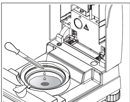
Wet the specimen sample with a few drops of water, so that the displayed weight is at least 0.5 grams (required minimum weight of sample).
