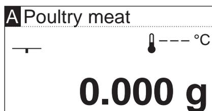
If you have saved the new method allocation, the chosen method will then be made available when you press the «A» key.
