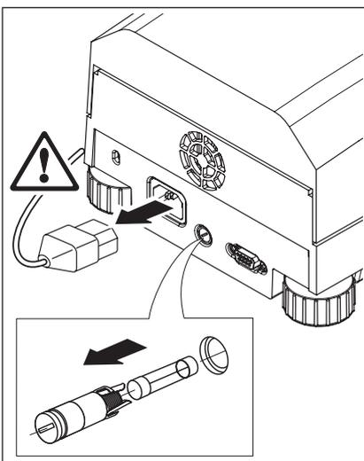
The power line fuse is located on the back of the instrument. Using a screwdriver, turn the fuse holder anticlockwise and pull it out of the instrument.
