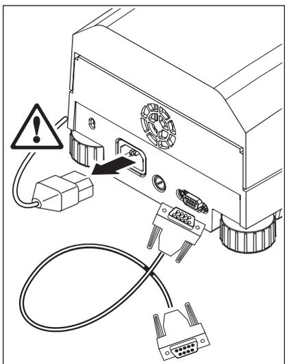
Connect the printer. The HB43-S is fitted with a 9-pin (f) socket for this purpose. The METTLER TOLEDO RS-P42 and RS-P26 plain paper printers are provided with suitable connection cables.
