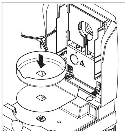
First lay the heat shield in the sample chamber. Then place the draft shield (can only be mounted in one position) and after that the sample pan support in position. Turn the sample pan support until it engages. In the engaged position the rear arm of the sample pan support lies exactly along the length of the instrument.
