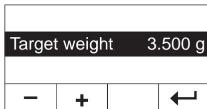
The current target weight flashes. You can use the «+» and «-» keys to change the weight in 0.5 g increments. The minimum value is 0.5 g, the maximum 54.0 g.
