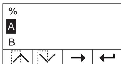
The existing name is deleted and the cursor is on the first character of the new name. Scroll the list of characters upwards or downwards until the required first character of the new name is displayed and press the «->» key to move the cursor to the next position. Choose the second character from the list of characters. The name of the method can be up to 20 characters long.
