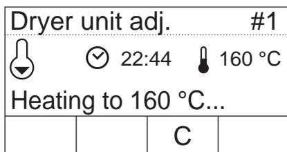
As this adjustment is a two-point adjustment (adjustment of the temperature is defined by two points, namely 100 °C and 160 °C), the heating module now heats to the second temperature (160 °C). Proceed exactly as you did for the first temperature. After you have confirmed your entry with «», the adjustment is at an end and the instrument automatically quits the menu and returns to the standby mode.
