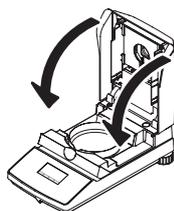
Close the heating module to start the adjustment process, and the heating module adjustment will begin.
