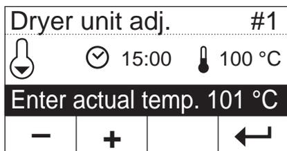
Read the temperature adjustment set through the inspection window of the heating module (the divisions correspond to 2 °C). Enter this temperature using the «+» and «-» keys. After entering the value, press «». The temperature must be entered within 10 minutes after the start of the beep, otherwise the adjustment process will be terminated and an error message output.
