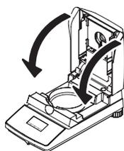
Close the heating module. The built-in balance is then automatically set to zero.
