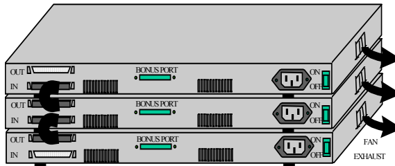
Figure 2.7b Magnum 8000X's stacked. Cables connect “Out” and “In”
