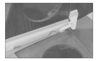
☐ Install the control horn to the left side of the rudder, making sure that the pushrod attachment holes are positioned over the rudder hinge line and that the control horn is lined up with the pushrod wire. The centerline of the control horn should be approximately 3/8" up from the bottom of the rudder, at the hinge line.
