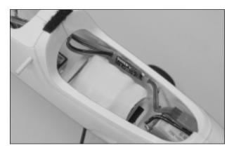
☐ Firmly stick the strip of Velcro® to your flight battery and secure the flight battery to the plywood mounting plate in the fuselage.
