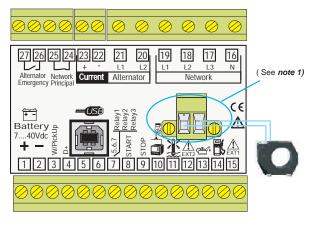
note 1: Connector only in Earth leakage protection option Dferencial.
