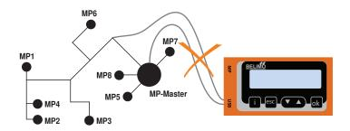
Solution: Use the service socket on the actuator or temporarily disconnect the MP connection of the MP device from the MP-Bus and connect the ZTH EU to the MP connection.
