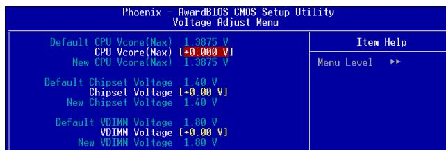
In the following items, "Default Voltage" indicates the original factory value, and "New Voltage" indicates the value that you assign.
