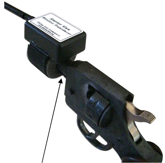
Barrel of Starting Pistol inserted into foam "Barrel Sleeve" of Transducer
