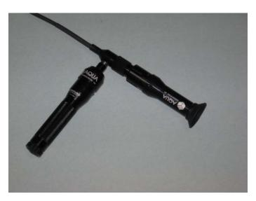
c. Attach the optional right angle mirror to the tip of the fiberscope if needed.
