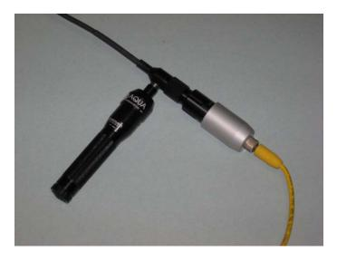
i. Connect the SnakeEye 4 foot cable to the SnakeEye display
