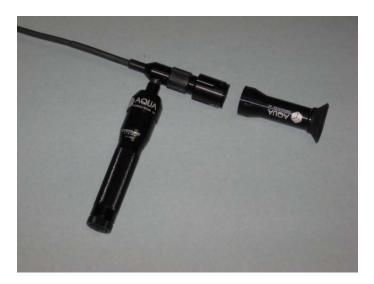
b. Connect the eyepiece (figure b.) to the fiberscope.
