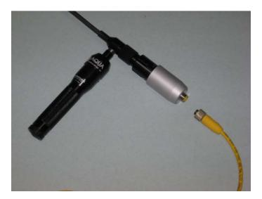
h. Connect the SnakeEye 4 foot cable to the C-mount camera.
