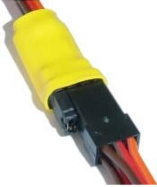
Figure 2. Programming mode - Jumper ON.
