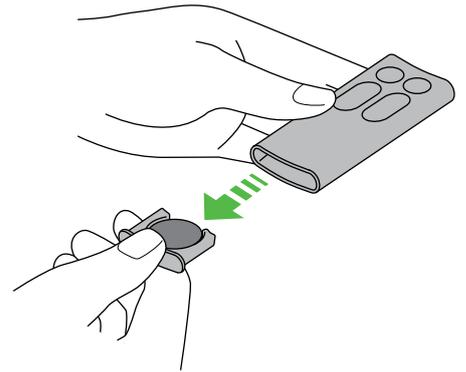
Press the end of the remote to release the battery.
