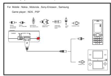
4) After fully charged the selected devices, unplug the cables and switch the button back to the "Charger" position. RED LED light will turn off immediately and the output process will be stopped. For safety reason, please take off the batteries from the C-514 charger after used.
