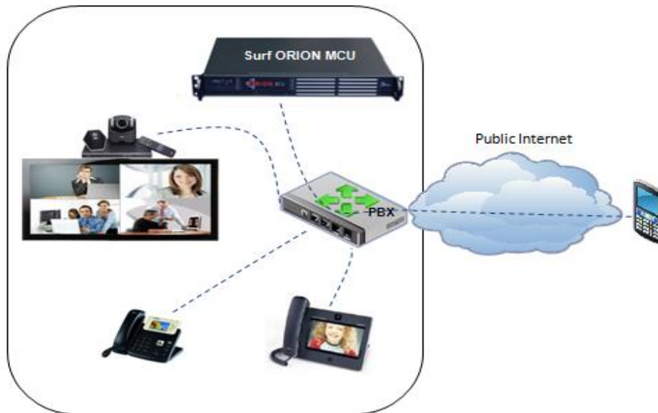
Figure 3-4: Topology 4 - Connectivity with External Networks
