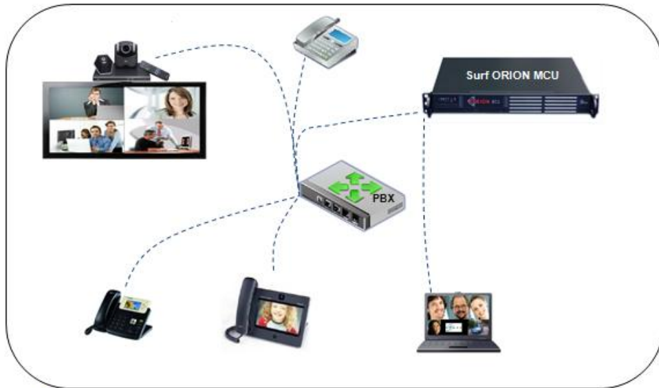
Figure 3-2: Topology 2 - Orion-MCU via PBX and Direct Connectivity
