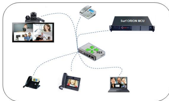
Figure 3-1: Topology 1 - Orion-MCU via SIP PBX
