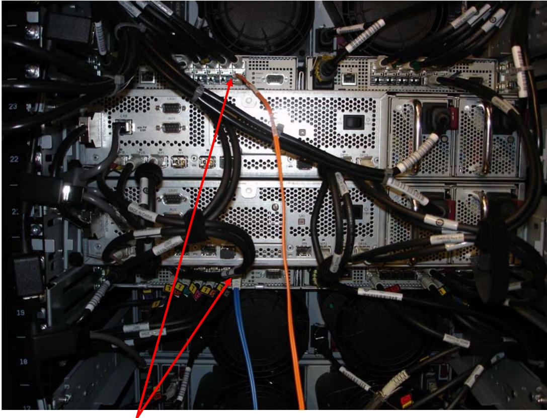
**View of Optical Connection to Tower Switches from Back of EVA5000**
