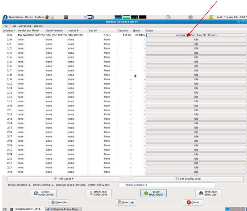
**Figure 3.6 – User Interface Screen Shows Purge Process Status**
