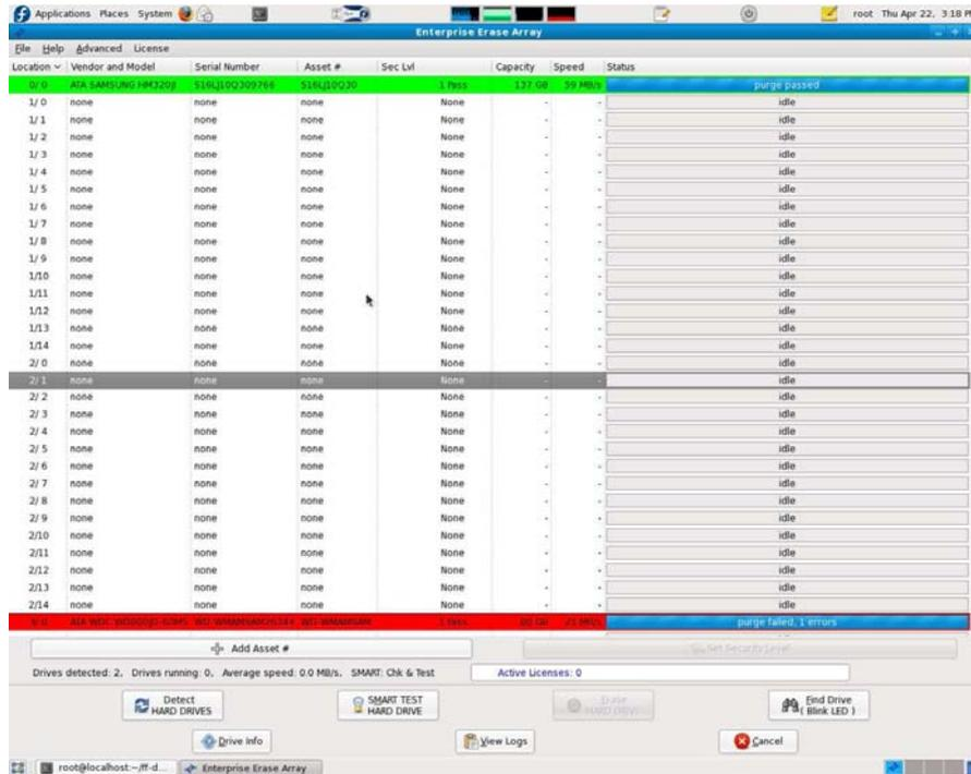
**Figure 3.7 – Successful Completion of Purge Process (Green Bar)
