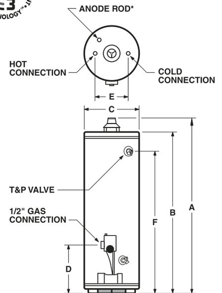
\*Location for optional top-mounted T&P Valve, if ordered from factory. To order, add "G" to model number (GS6 40 YBRTG).
